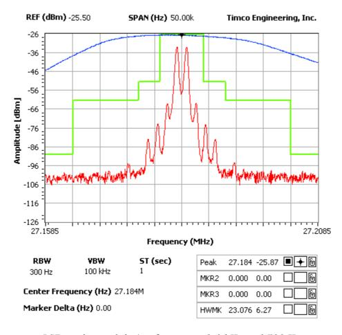
LSB mode: modulation frequency 2.4 kHz and 500 Hz
