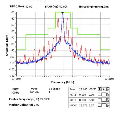
AM mode: modulation frequency 2.5 kHz
