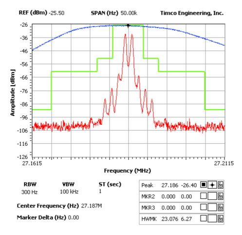
USB mode: modulation frequency 2.4 kHz and 500 Hz
